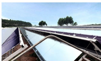
Mirror-Array unit in double-gain mode
